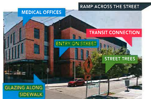
Example of an office building that creates a walkable environment with its ground-floor elements and landscaping.
